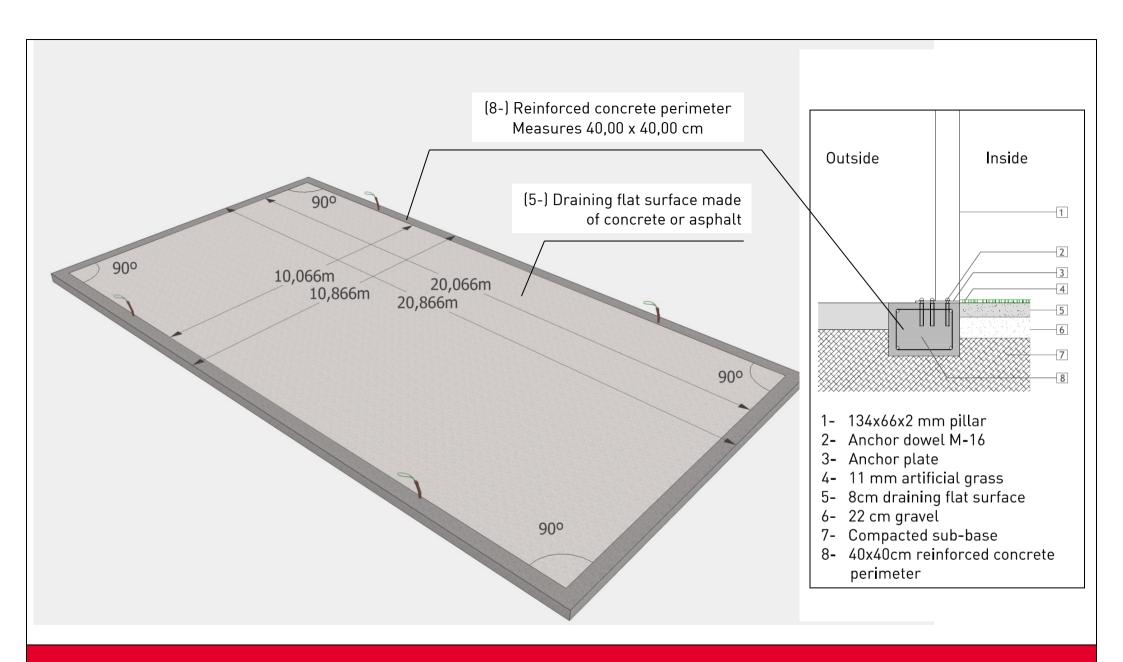
01. Before Padel court installation: Staking inner rectangle paddle court of 20,066 m x 10,066 m, with a width of 40 cm bands.
